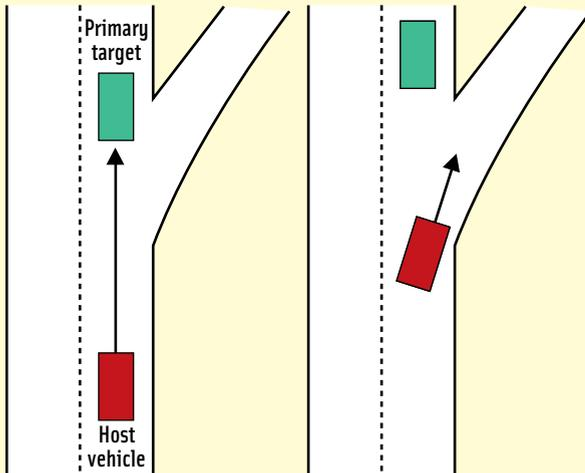
FIGURE 4 Using the ramp map database attribute for the ACC system.
